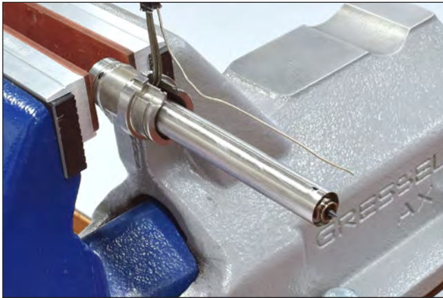
Picture 87: Disassemble the broken thermocouple
