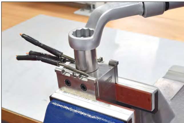
Picture 98: Clamp the nozzle and unscrew the adapter
