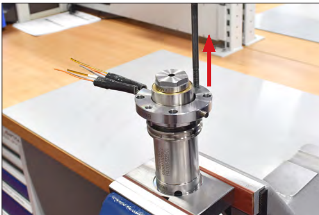
Picture 113: Dismantle hold-down device
