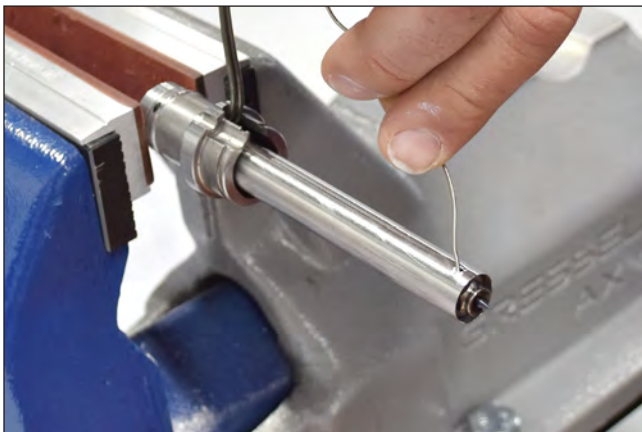
Picture 89: Installation of the new thermocouple
